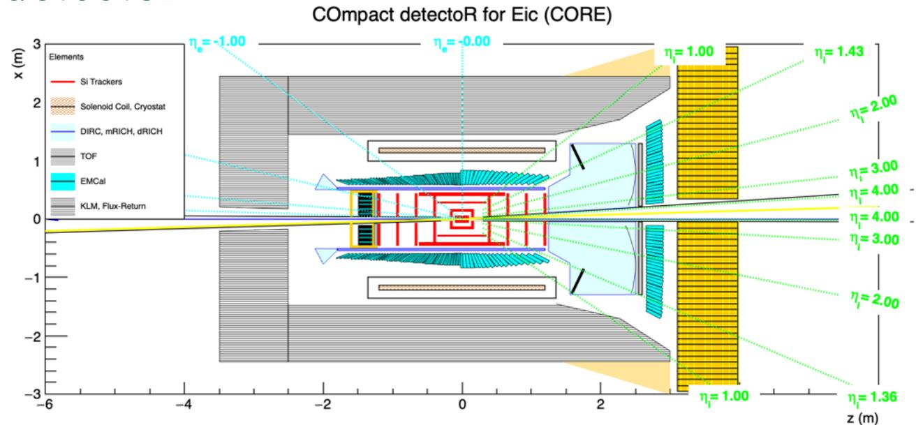
A short solenoid is essential for reaching the highest luminosity on day 1, and offers a potential for future upgrades (magnets can be moved in further if optical meta materials can replace dRICH gas)
