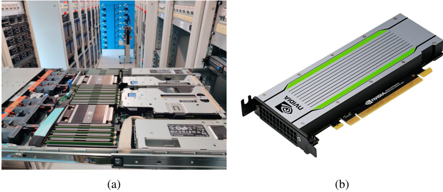
Figure 2: (a) Single HLT Node for Run-3, equipped with two AMD Milan 64-core CPUs and two NVIDIA T4 GPUs. The HLT Farm for Run-3 has 200 nodes. (b) NVIDIA T4 GPU.
