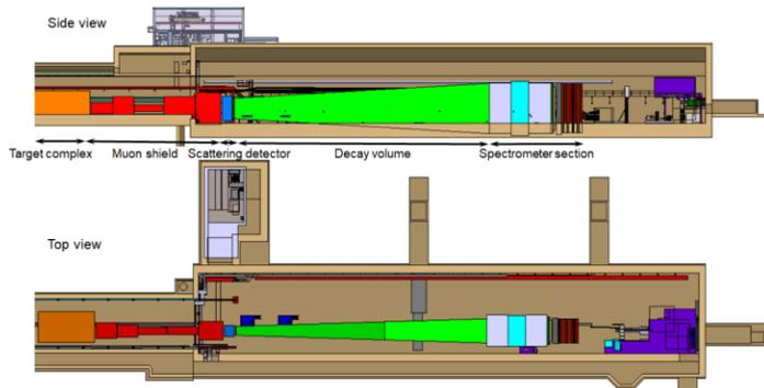
**Figure 1.** Views of the SHiP ECN3 option. Top view shows the ground profile along the relevant section of TCC8 and ECN3. The two bottom views shows a preliminary integration of the SHiP detector [7].
