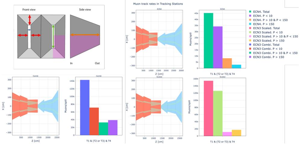
**Figure 3.** Front and side view of the shield magnet (on the top-left). All unique parameters are marked by the arrow of a different color. Manually adapted Muon Shield and corresponding metrics (on the right).
