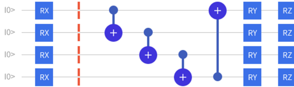
Figure 4: The schematic diagram of the quantum convolutional kernel. "RX", "RY", and "RZ" represent single-qubit rotation gates around the X, Y, and Z axes, respectively, while " \oplus " represents the CNOT gate with entanglement operation.
