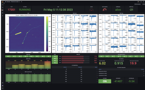
Figure 3. The CYGNO remote console available for user following the run from remote - without the need to access the DAQ, restricted to experts - where the following are available: device setting and readout, sample of raw images collected and PMT waveforms, typically updated every 5 seconds.
