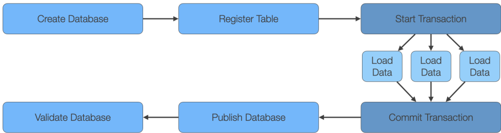
Figure 3: Schematic view of the data ingestion process into Qserv database.
