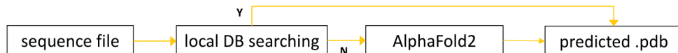
Figure 2. Scenario B: predicted using AlphaFold2 workstation that is usually with high accuracy but at slow speed.
