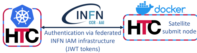
Figure 4: Detached HTCondor submit node running in a remote Docker container.
