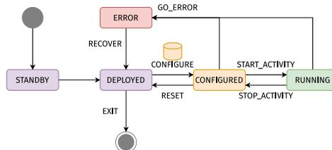
**Figure 3.** The state machine of an AliECS environment. The same state machine is implemented by each task. For FairMQ-based tasks the OCC plugin acts as a translation layer between the AliECS task state machine and the underlying FairMQ state machine.
