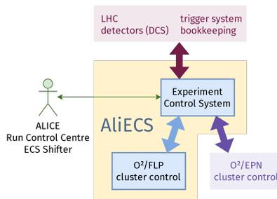
**Figure 1.** O<sup>2</sup>/FLP and O<sup>2</sup>/EPN cluster control with respect to the ALICE Run Control Centre.
