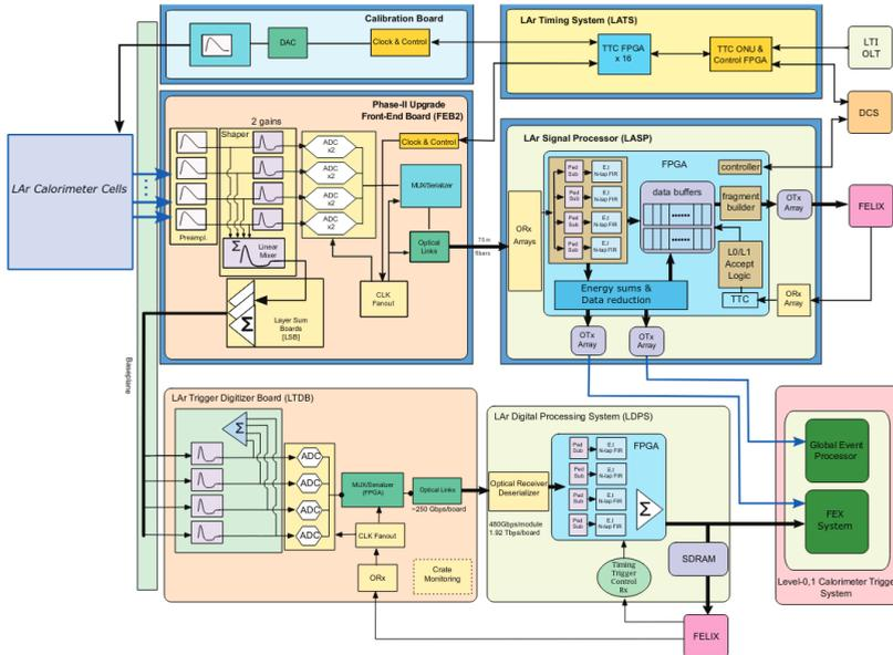
**Figure 1.** LAr calorimeter readout upgrades for HL-LHC era. Calibration, Front-End and Signal Processing boards are under development for the Phase-II upgrades covered in this document.
