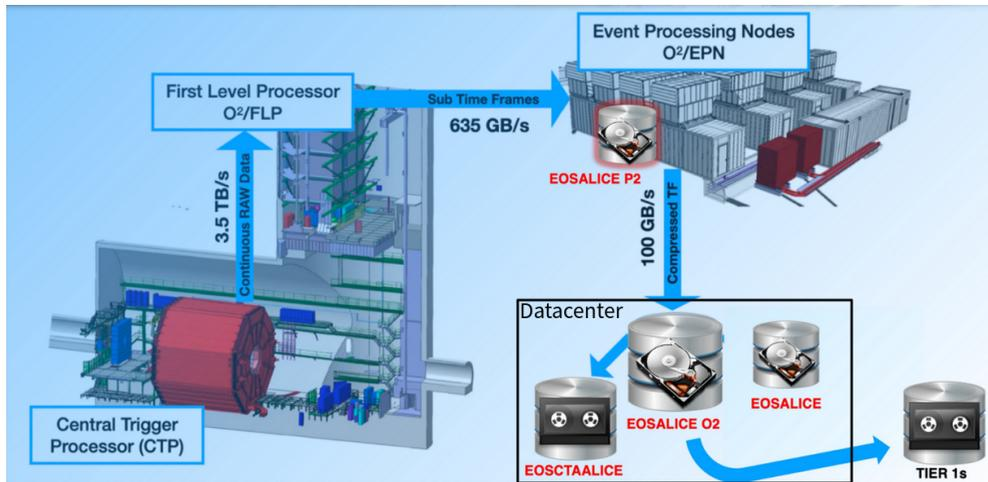
Figure 4: The ALICE experiment data taking workflow
