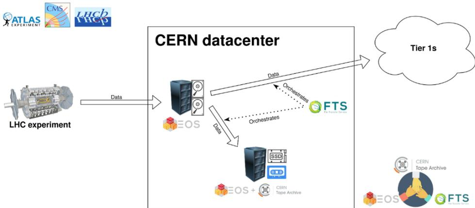
Figure 3: The General LHC experiments data taking workflows using EOS, CTA and FTS
