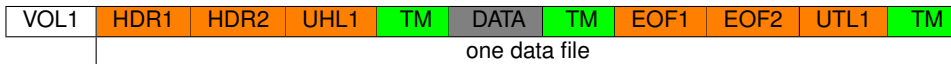
Figure 2: ANSI AUL tape data format [11] used by CASTOR/CTA, with descriptors for volume label (VOL1), headers (HDR), user headers/trailers (UHL/UTL), end-of-file (EOF); tape marks (TM); and the payload (DATA). Descriptors are stored in tape blocks of 80 bytes; for more details see [12].
