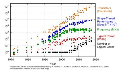
Break down of DS (leakage current), Moore's Law (atom sized devices), CS (too much power)
