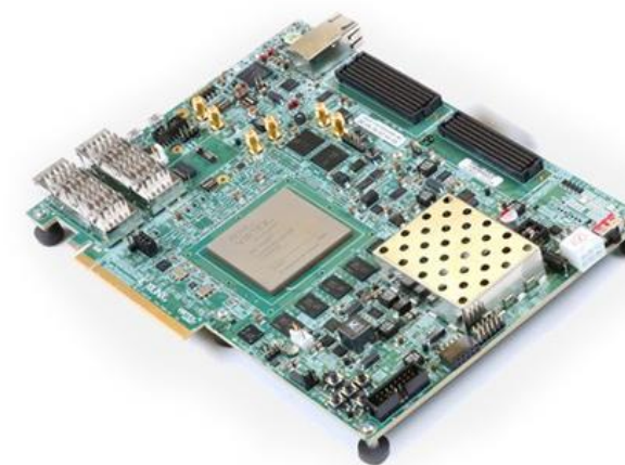
Fig5: The FPGA for testing design
