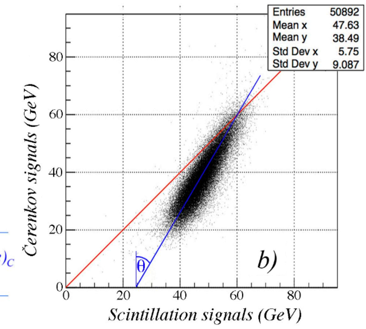
b) Scatter plot of C and S signals for 60 GeV pions in the RD52 lead-fiber calorimeter
