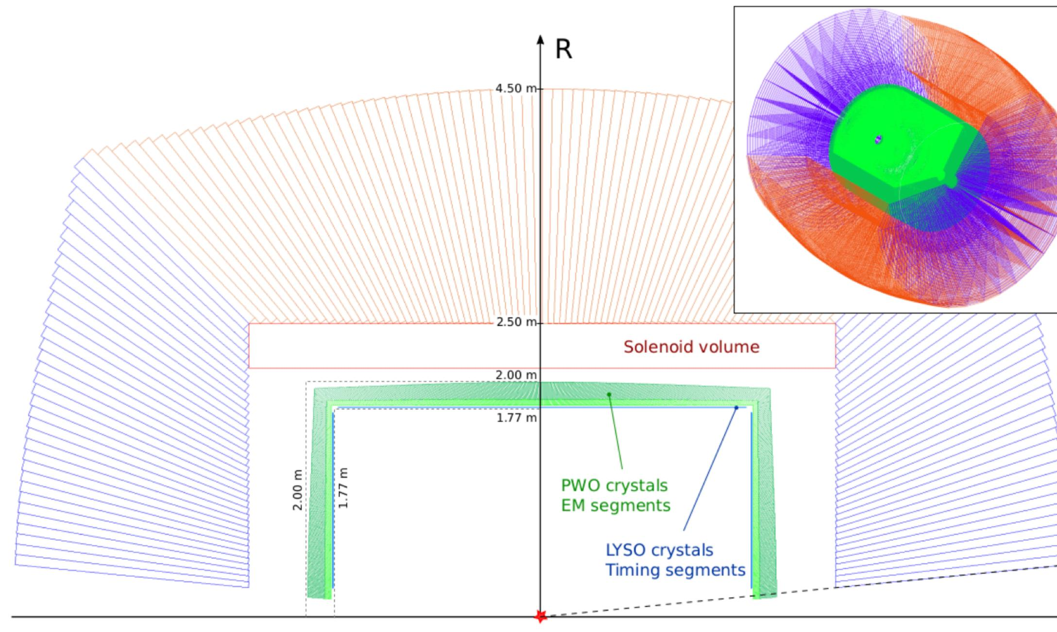
Integration of a crystal calorimeter option in the GEANT4 IDEA simulation:
