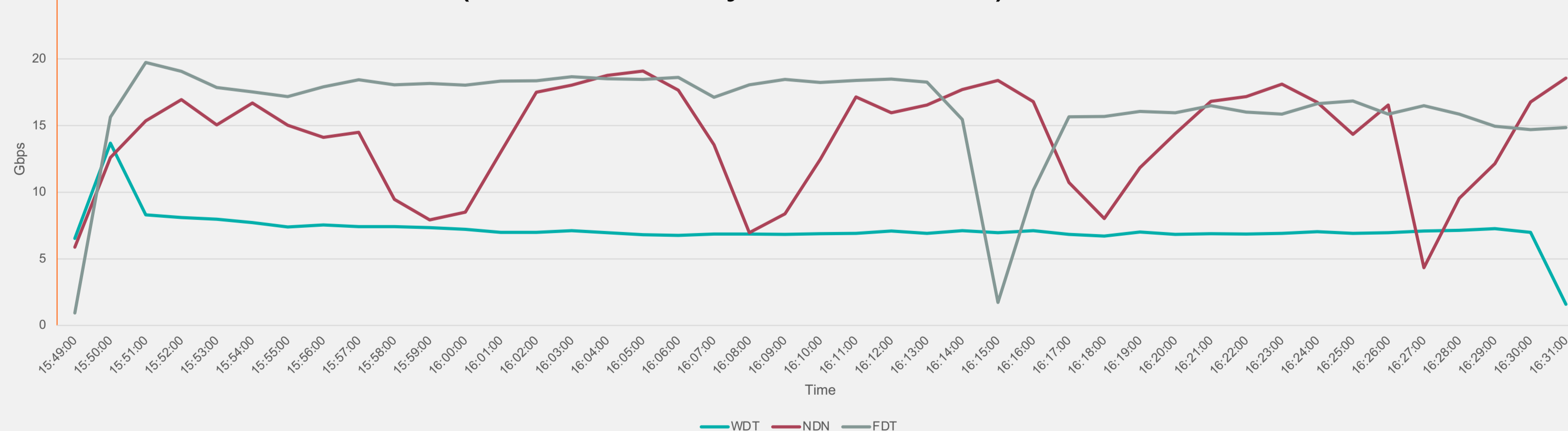
Fig 4. Multi Threaded WAN Transfer (75ms latency, 16 threads)
