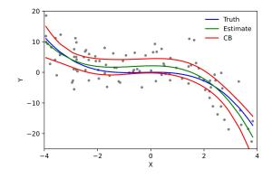
Example of a cubic polynomial regression, which is a type of linear regression. Although *polynomial regression* fits a nonlinear model to the data, as a statistical estimation problem it is linear, in the sense that the regression function  $E(y \mid x)$  is linear in the unknown parameters that are estimated from the data. For this reason, polynomial regression is considered to be a special case of multiple linear regression.
