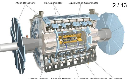
Toroid Magnets Solenoid Magnet SCT Tracker Pixel Detector TRT Tracker
