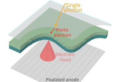
Development of a new photodetector with large active area able to measure single photons with simultaneous excellent timing and spatial resolution, with a low noise
