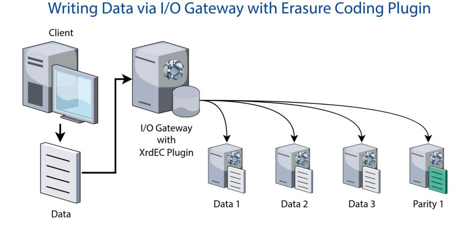
When reading, the data can be reconstructed either at the server, in case the client does not have support for erasure coding enabled, or each block can be read directly if the client has support for erasure coding enabled. The client can also write data directly in this case.
