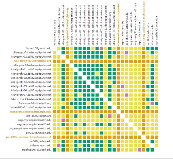
Throughput >= 30Gbps Throughput >= 10Gbps Throughput < 10Gbps Unable to retrieve data Check has not yet run Down for maintenance
