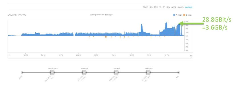
Dedicated OSCARS link between CERN and Fermilab. Blue is CERN->Fermilab, Orange is Fermilab->CERN We had enough network and transfer bandwidth to do the data challenge and still take raw data on the cold box.
