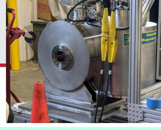
New solenoid on loan to MOLLER collaboratio for Kerr Effect measurements.
