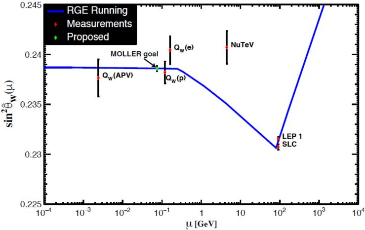
•  $\sin^2 \theta_W$  is precisely given by Standard Model and anchored by the Z-pole measurements, LEP1 & SLC
