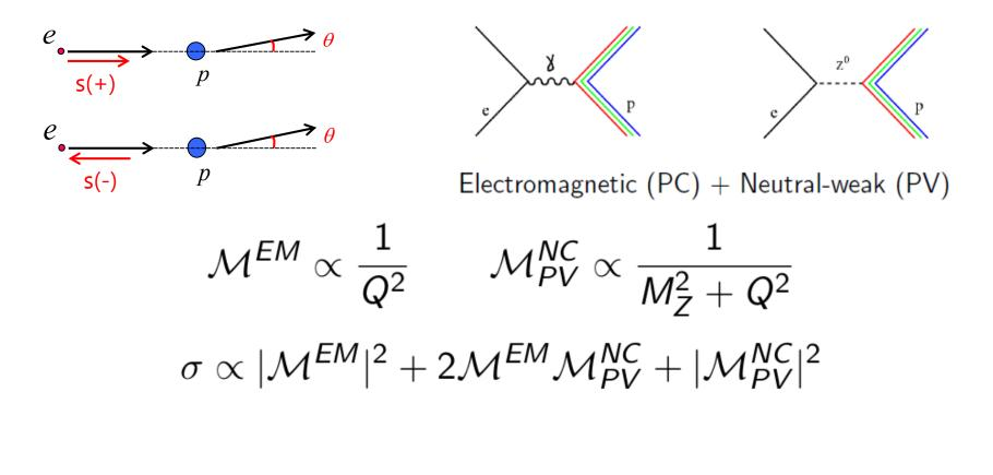
$$A_{PV}(p) = \frac{\sigma_R - \sigma_L}{\sigma_R + \sigma_L} \propto \frac{\mathcal{M}_{PV}^{NC}}{\mathcal{M}^{EM}} \propto \frac{Q^2}{M_Z^2} \quad \text{when } Q^2 \ll M_Z^2$$
