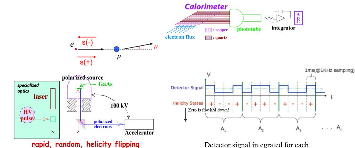
Detector signal integrated for each helicity window and asymmetry formed from helicity patterns
