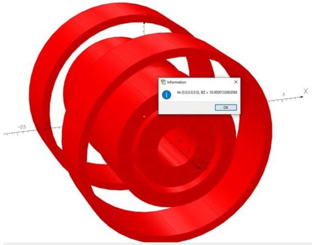
Coil configuration of a 16-T MRI Magnet
