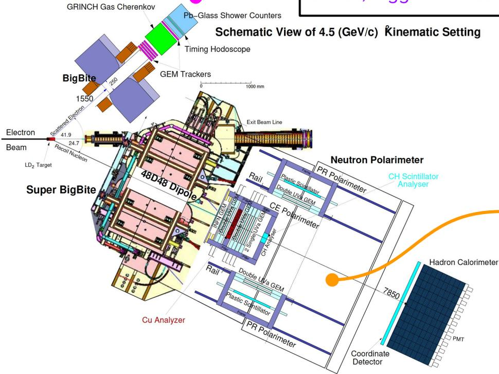
Neutron arm/Polarimeter (position, time-of-flight, and spin precession for recoiling nucleon):
