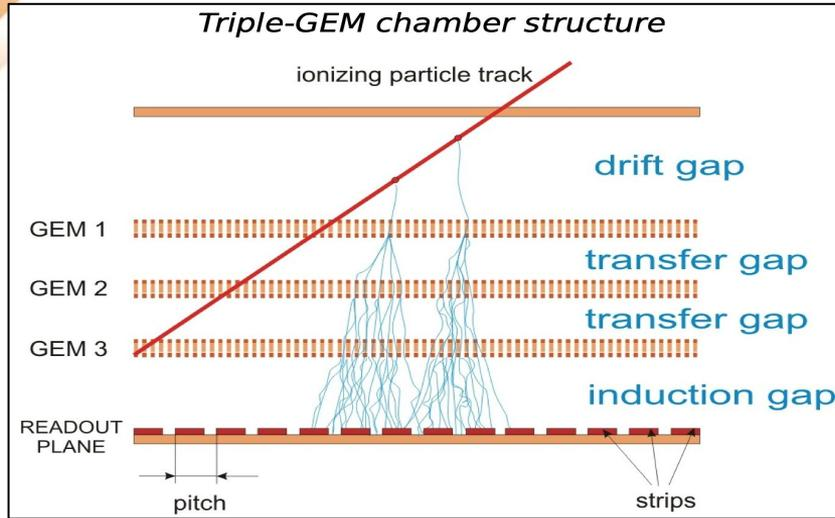
**GEM detectors:** cost effective solution for high resolution tracking under high rates over large areas.
