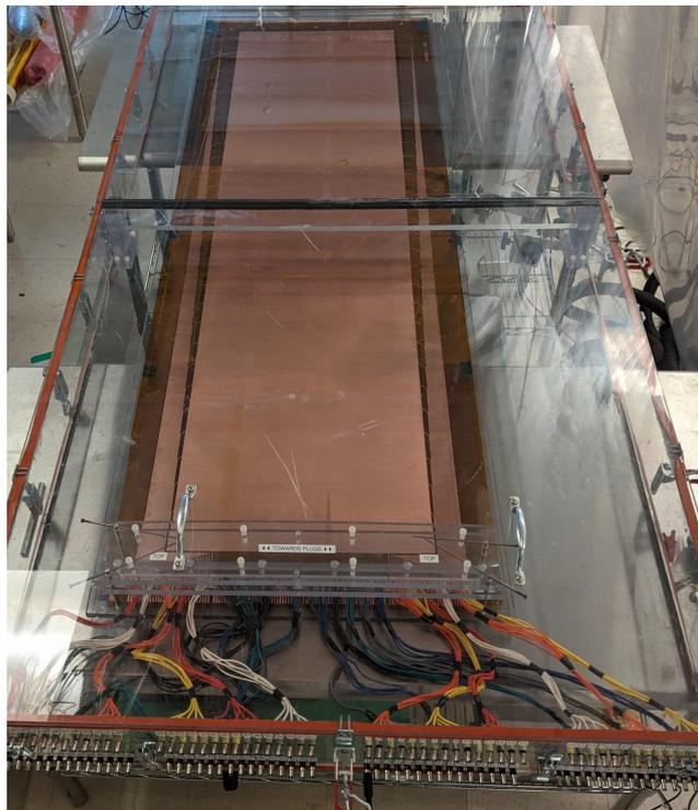
Testing a UV GEM foil under high voltage in a dry nitrogen environment
