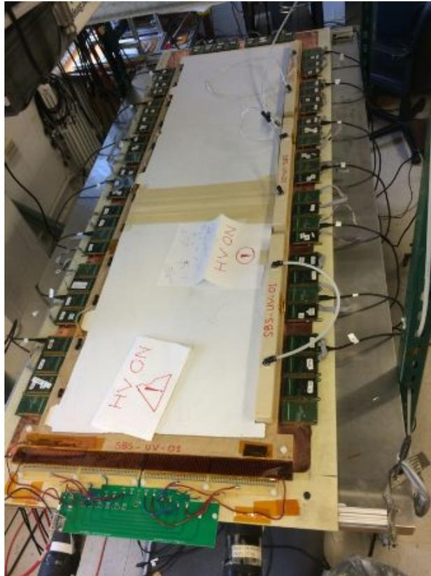
Completed UV chamber on cosmic test stand
