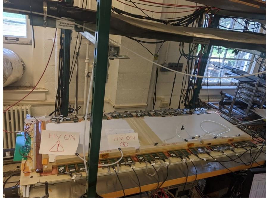
Assembled UV GEM Chamber on a cosmic test stand
