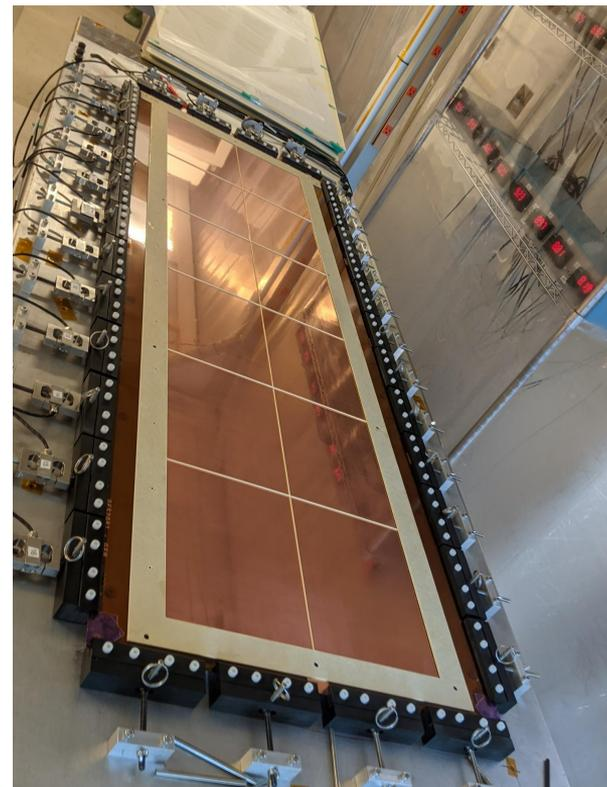
UV frame installed onto a mechanically-stretched GEM foil
