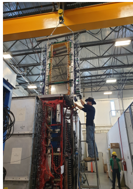
Figure: Inserting a GEM layer into the Bigbite electron spectrometer
