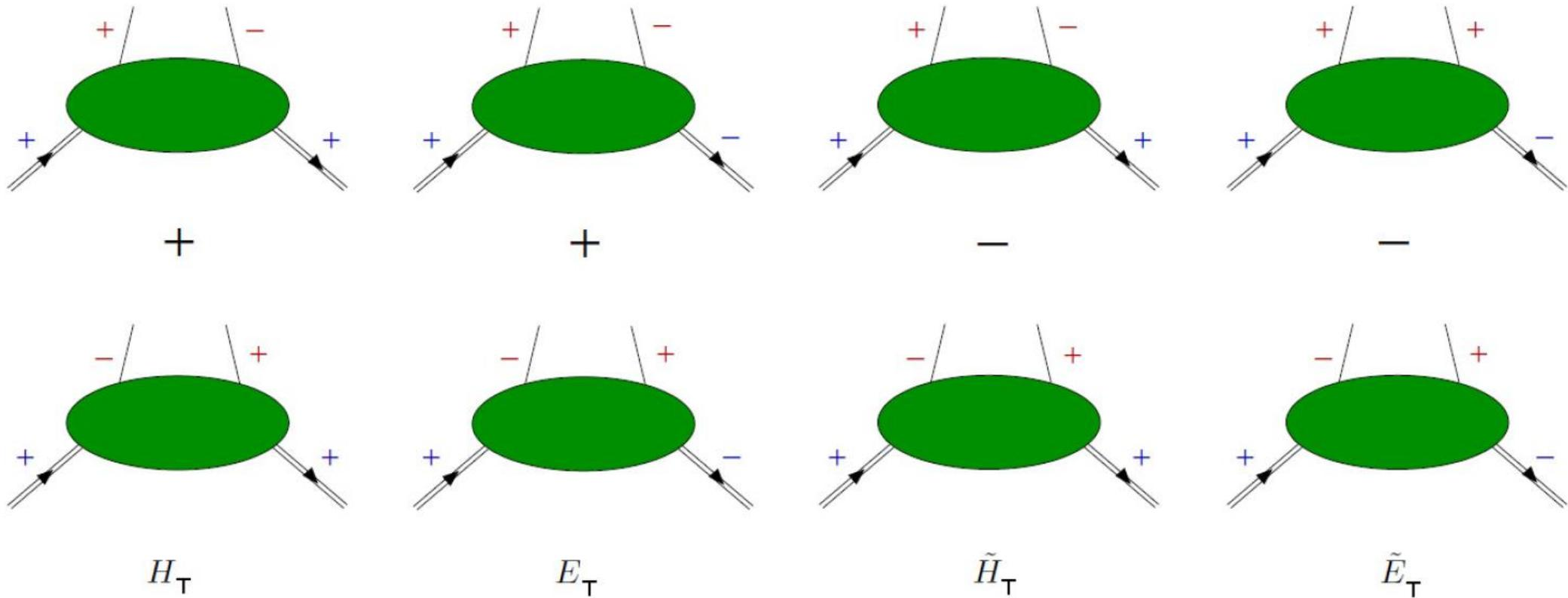
4 chiral-odd GPDs: flip helicity of the quark
