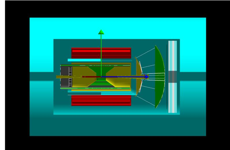
CORE with a gas-only RICH (eRD6) and LGAD-based TOF behind it
