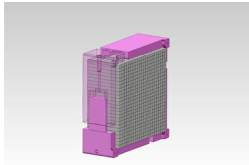
The CMS PWO pre-shower uses cooled 6 mm Si-strip detectors in-between an initial layer and the main PWO blocks
