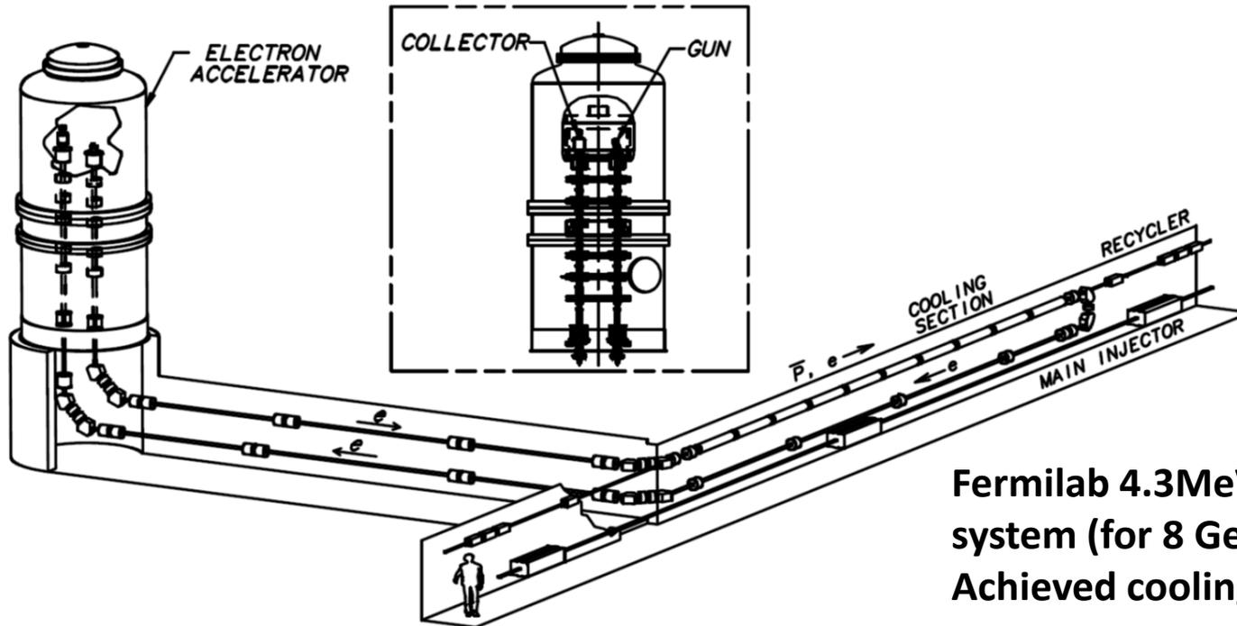
Fermilab 4.3 MeV electron cooling system (for 8 GeV antiprotons)
