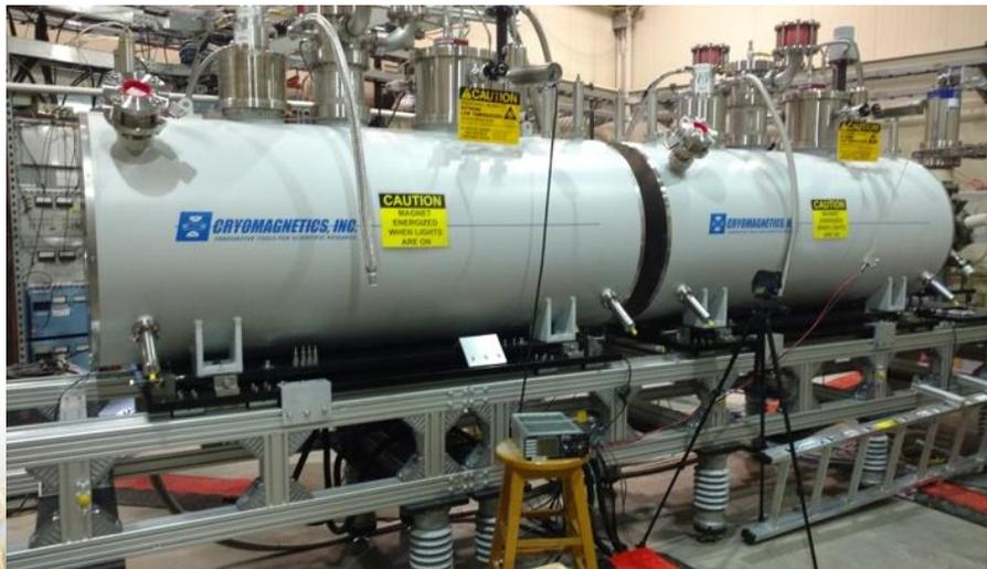
Electron beam ion source
