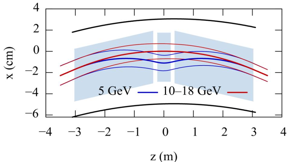
Super bends: Electron Storage Ring arc dipoles split into 3 segments
