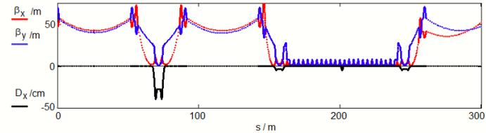
Figure 2: Electron beam optics in the cooling section
