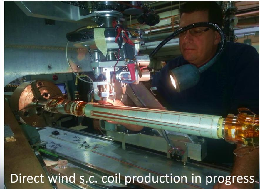
Direct wind s.c. coil production in progress
