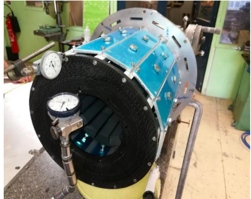
Artefact scintillator modules with similar weight to evaluate the deformation of the structure
