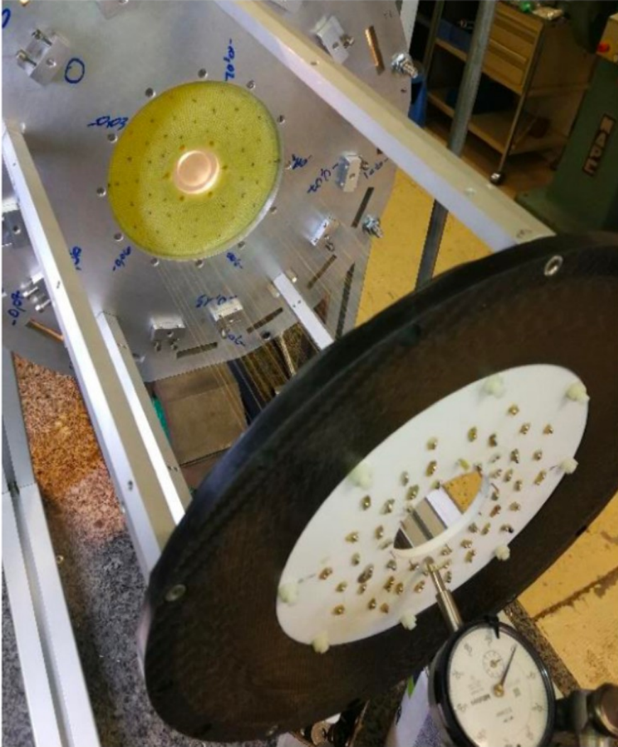
Tungsten wires to simulate the tension due to the 3026 aluminum wires (36 Kg)
