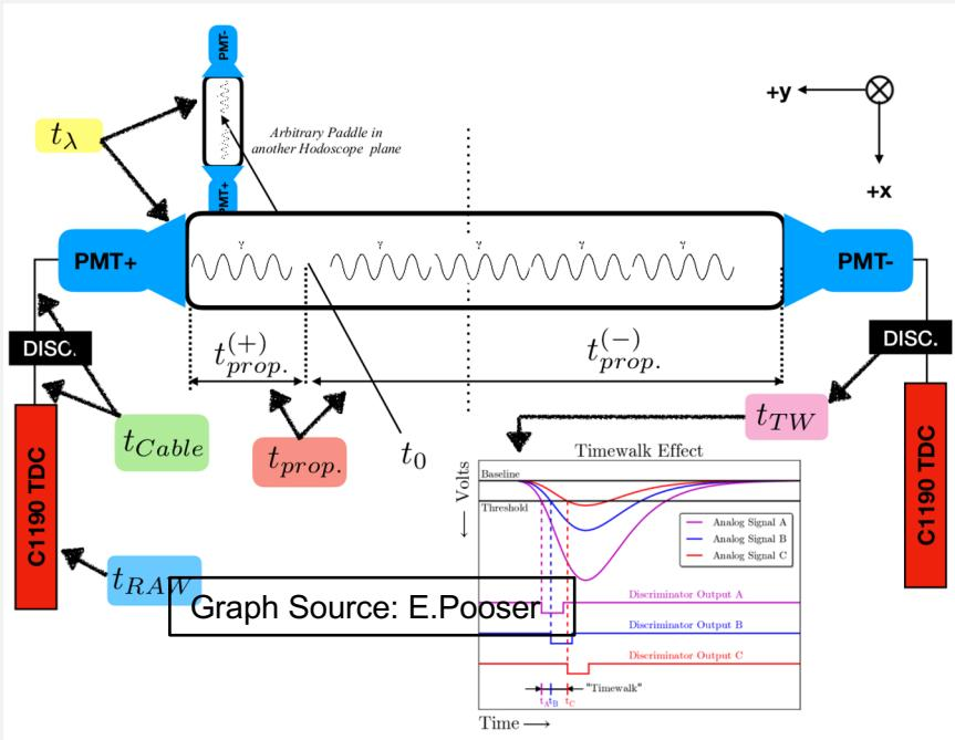
$$t_{Corr} = t_{RAW} - t_{TW} - t_{Cable} - t_{propagation} - t_\lambda$$
