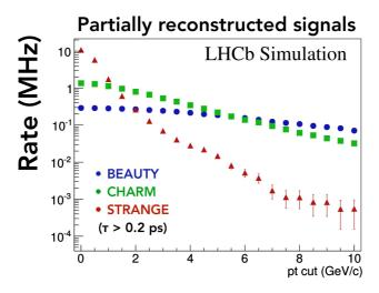
30 MHz (4 TB/s) of input contains a MHz of signal, while we can only store 10 GB/s long-term
