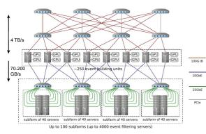
GPU solution (Allen) selected as baseline HLT1; up to 3 GPUs installed in each event builder server
