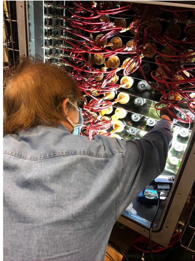
Applying UV curing light to cure the epoxy
