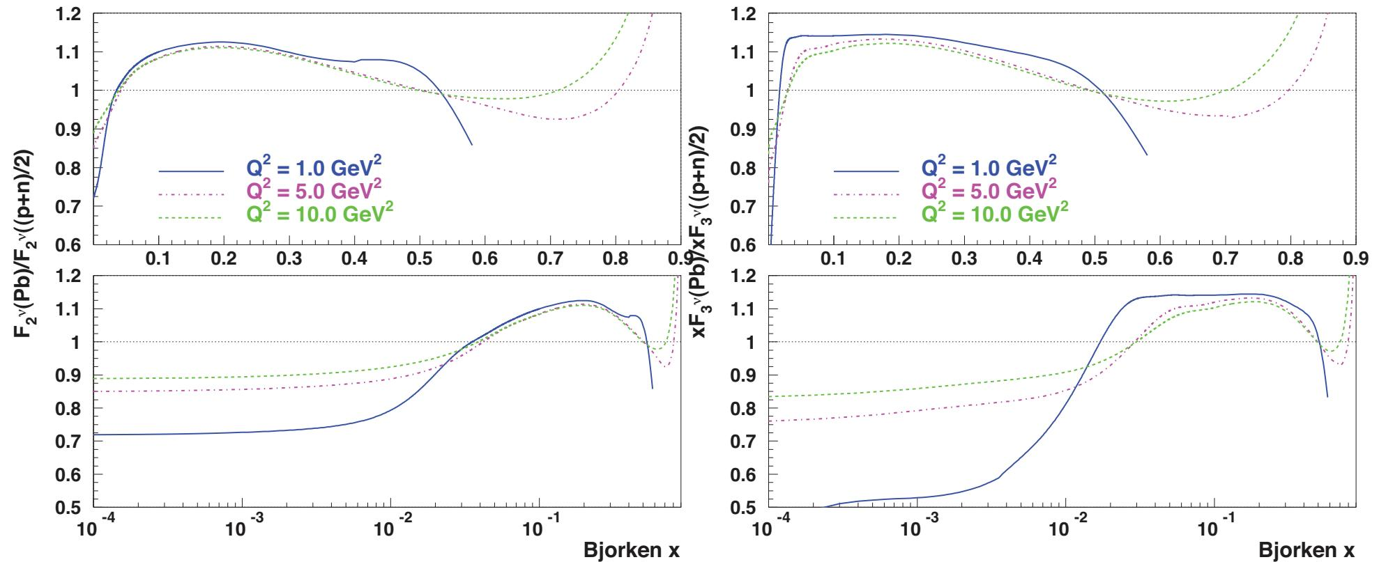
*Ratio of Charged Current structure functions on  $^{207}\text{Pb}$  and isoscalar nucleon ( $p + n$ )/2*
