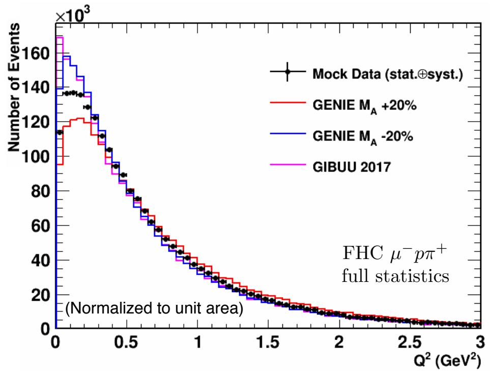
Expected  $Q^2$  distribution for  $\nu_\mu p \rightarrow \mu^- p\pi^+$  on H (5y low-energy beam)
