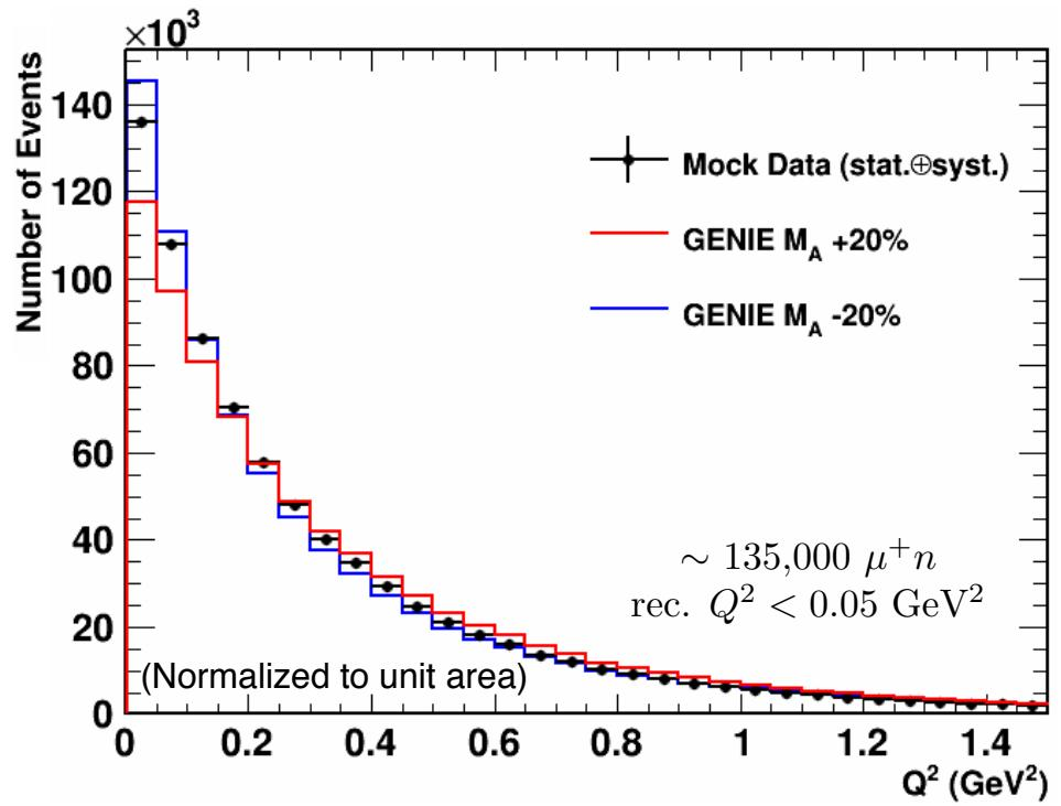
Expected  $Q^2$  distribution for  $\bar{\nu}_\mu p \rightarrow \mu^+ n$  QE on H (5y low-energy beam)
