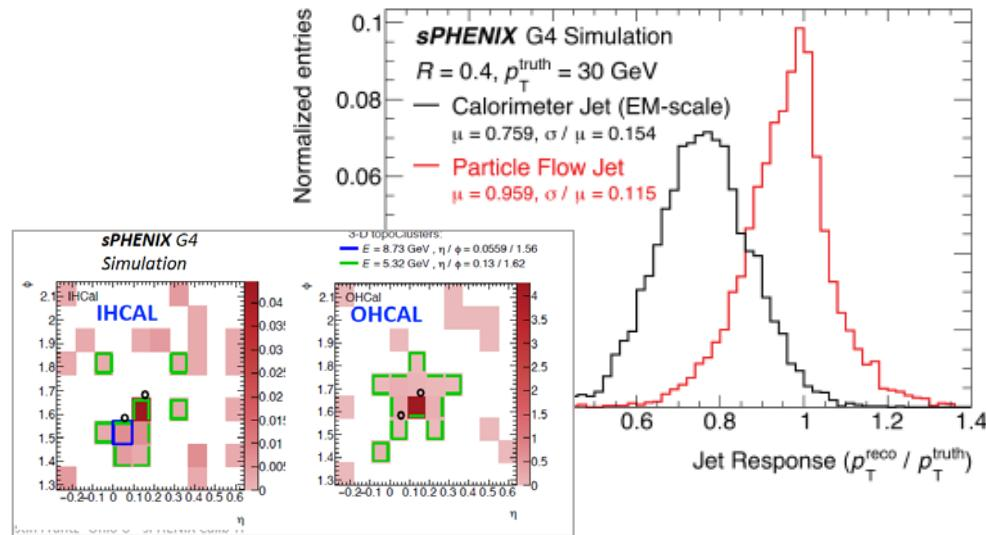
3D All-Calorimeter Clustering/Jet Particle Flow
