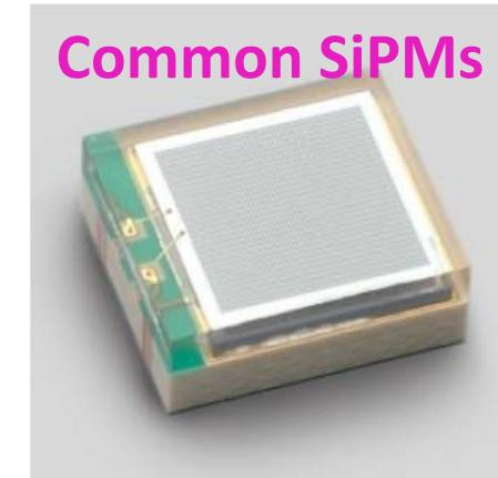
Figure 5.3: Hamamatsu S12572 MPPC (SiPM). The device is  $3 \times 3 \text{ mm}^2$  with 40,000 pixels  $15\mu\text{m}^2$ .
