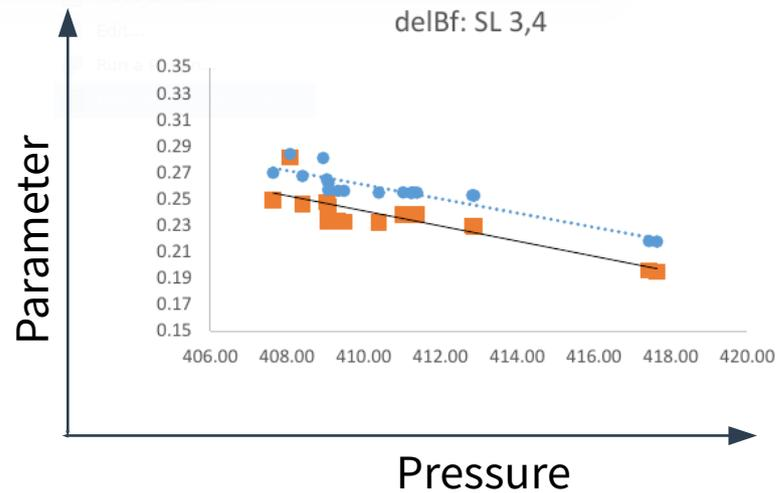
Linear dependence of the parameters on the atmospheric pressure
