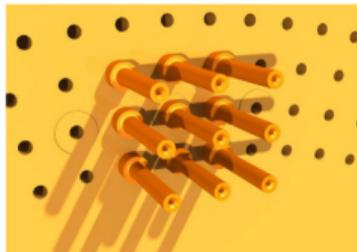
Wires are crimped to the PCB via feedthroughs
