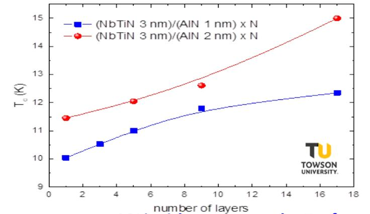
Metamaterial engineering shows hyperbolic behavior and increased the  $T_c$  of these multilayered structures up to 32% with respect to the  $T_c$  of a single ultrathin NbTiN layer. Enhancement limited by the small coherence length of NbTiN ( $\xi \sim 3.8$  nm).
