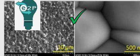
Modification of coating process based on learnings from correlated material and RF studies of Nb<sub>3</sub>Sn samples resulted in the removal of recurrent Q-slopes.
