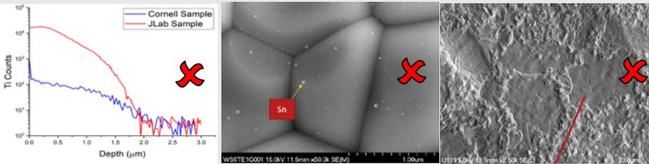
Potential factors contributing to recurrent Q-slopes in Nb<sub>3</sub>Sn cavities
