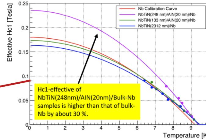
$H_{c1}$ -effective of NbTiN(248nm)/AlN(20nm)/Bulk-Nb samples is higher than that of bulk-Nb by about 30%.
