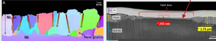
Grain-boundary diffusion primarily controls thin-film growth. Patchy regions lack grain boundaries resulting in RF-affecting thin regions.
