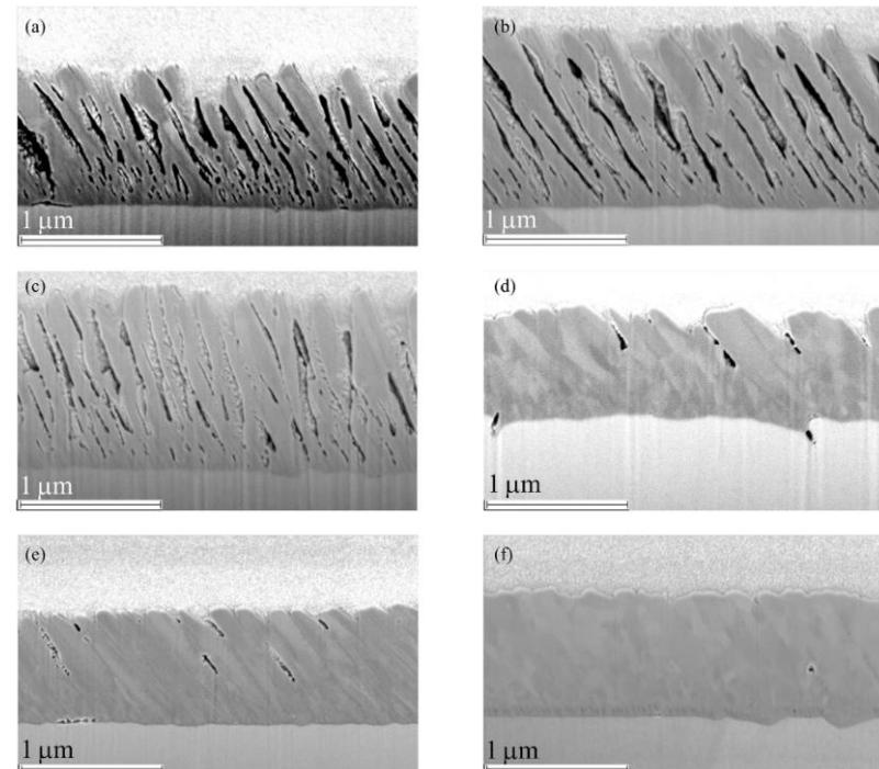
Fig. 5. Nb films FIB cross sections of samples at 90° coated in: (a) DCMS with grounded substrate, (b) DCMS with -50 V biased substrate, (c) HiPIMS with grounded substrate, (d) HiPIMS with -50 V biased substrate, (e) HiPIMS with grounded substrate and +50 V PP, (f) HiPIMS with grounded substrate and +100 V PP.
