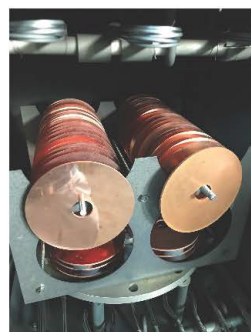
Figure 1: A picture of Cu (C1020) disks set in the vacuum furnace for annealing process.
