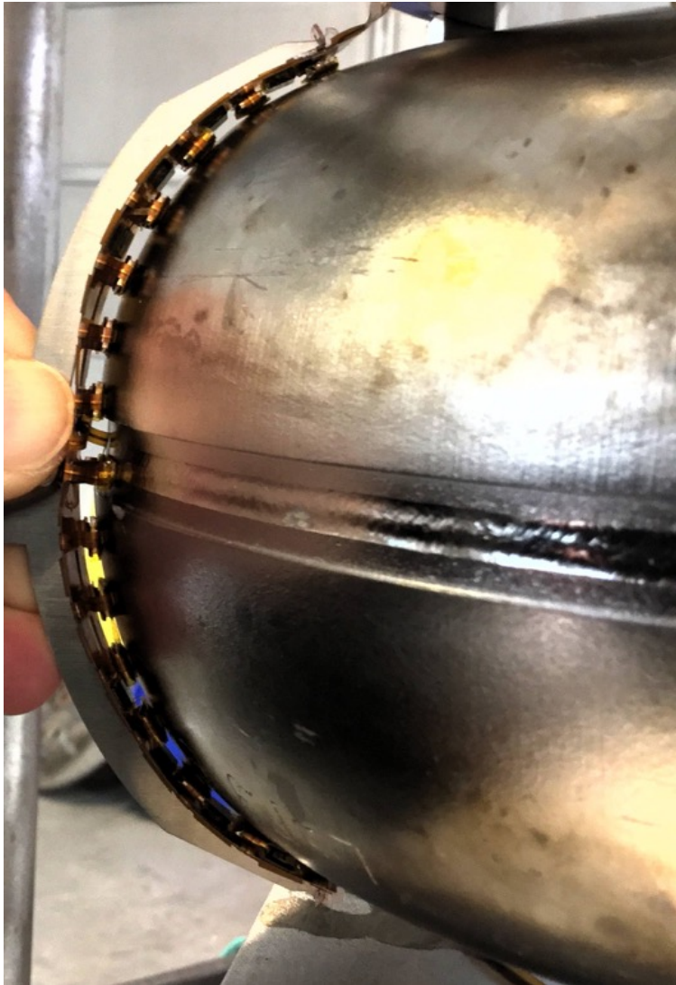
T-sensors fit on the cavity surface.
