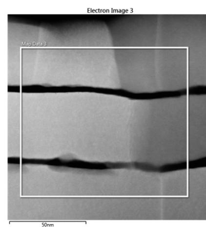
$\text{Al}_2\text{O}_3$  layer well-confined
