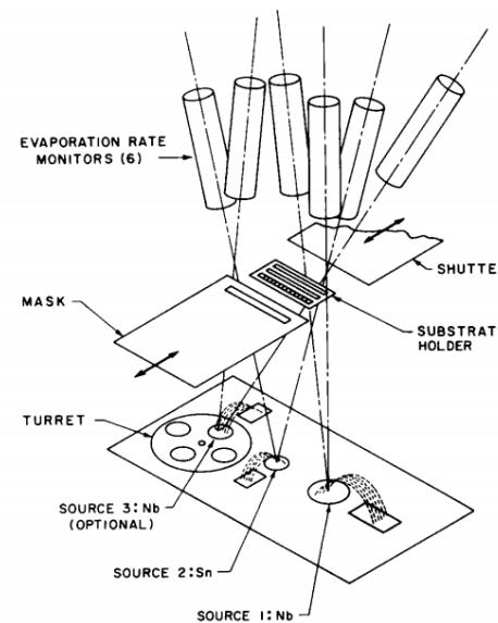
FIG. 1. Schematic of electron-beam deposition system showing linear source arrangement.
