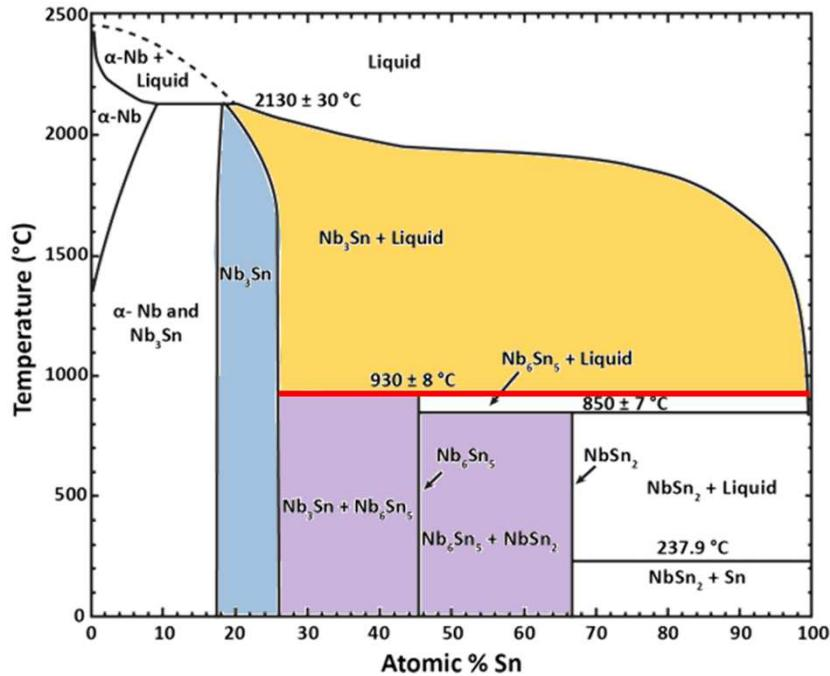
Below 930 °C: Nb<sub>6</sub>Sn<sub>5</sub>, NbSn<sub>2</sub> are stable
