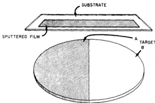
FIG. 1. The relative positions of the sputtering target and substrate.
