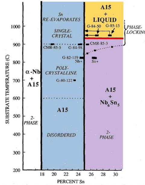
Fig. 1. A portion of the phase diagram for Nb-Sn showing the A15 phase field and adjacent regions. Italicized comments refer to the properties of films prepared in those regions, and the location of the dotted lines separating the regions are approximate. Samples discussed in this paper are marked at their deposition temperature and composition.
