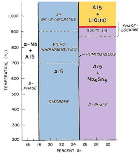
Fig. 2. A portion of the Nb-Sn phase diagram. The phase fields are labeled in large type and bounded by solid lines. The diagram is further divided into regions which are labeled in italics with a description of the main characteristic of thin films which are prepared there.
