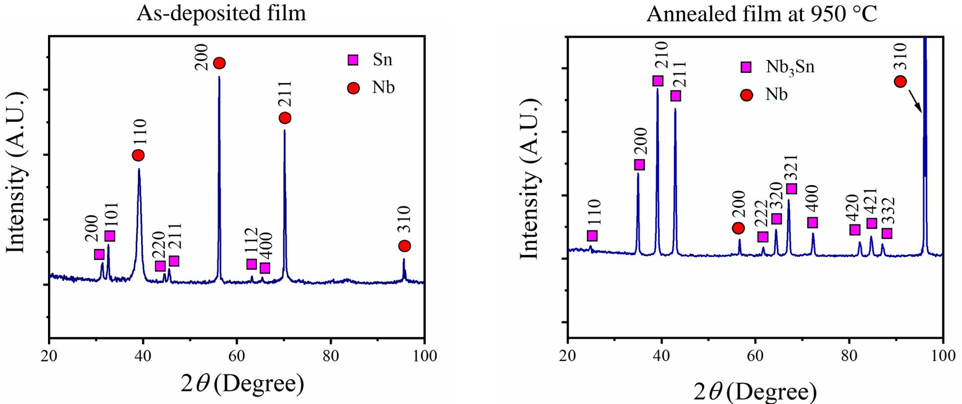
Figure: X-ray diffraction pattern of as-deposited and annealed films.
