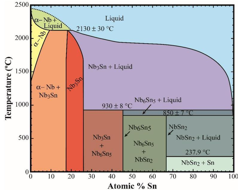
Binary phase-diagram of Nb and Sn, adapted from [1].
