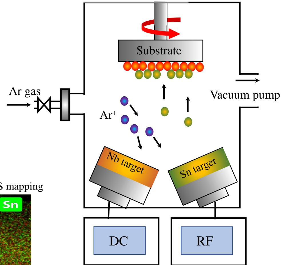
Figure: Schematic diagram of the sequential sputter deposition.
