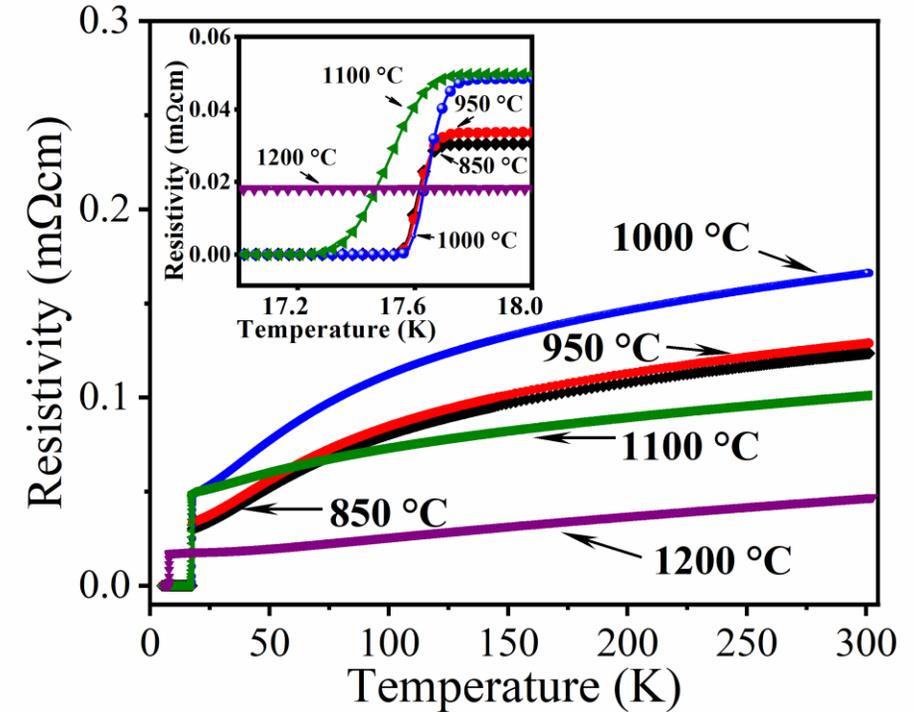
Figure: Resistivity vs temperature.
