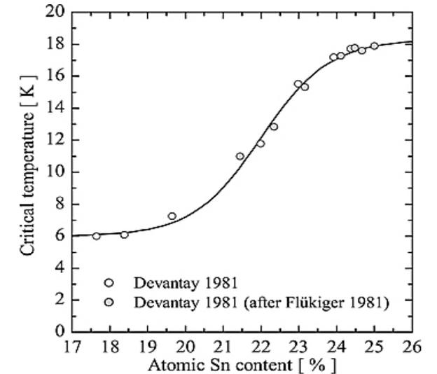
Critical temperature of Nb<sub>3</sub>Sn as a function of atomic Sn content [2].
