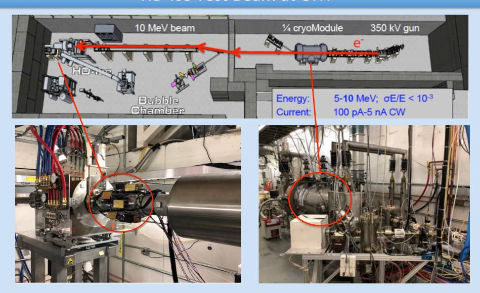
UITF beam line under commissioning: reached the target energy of 9.5 MeV New target ready. First beam through IBC (empty target) expected within September.
