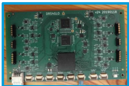
Precision timing digitizer DRS4GIO (SBIR/LDRD)
