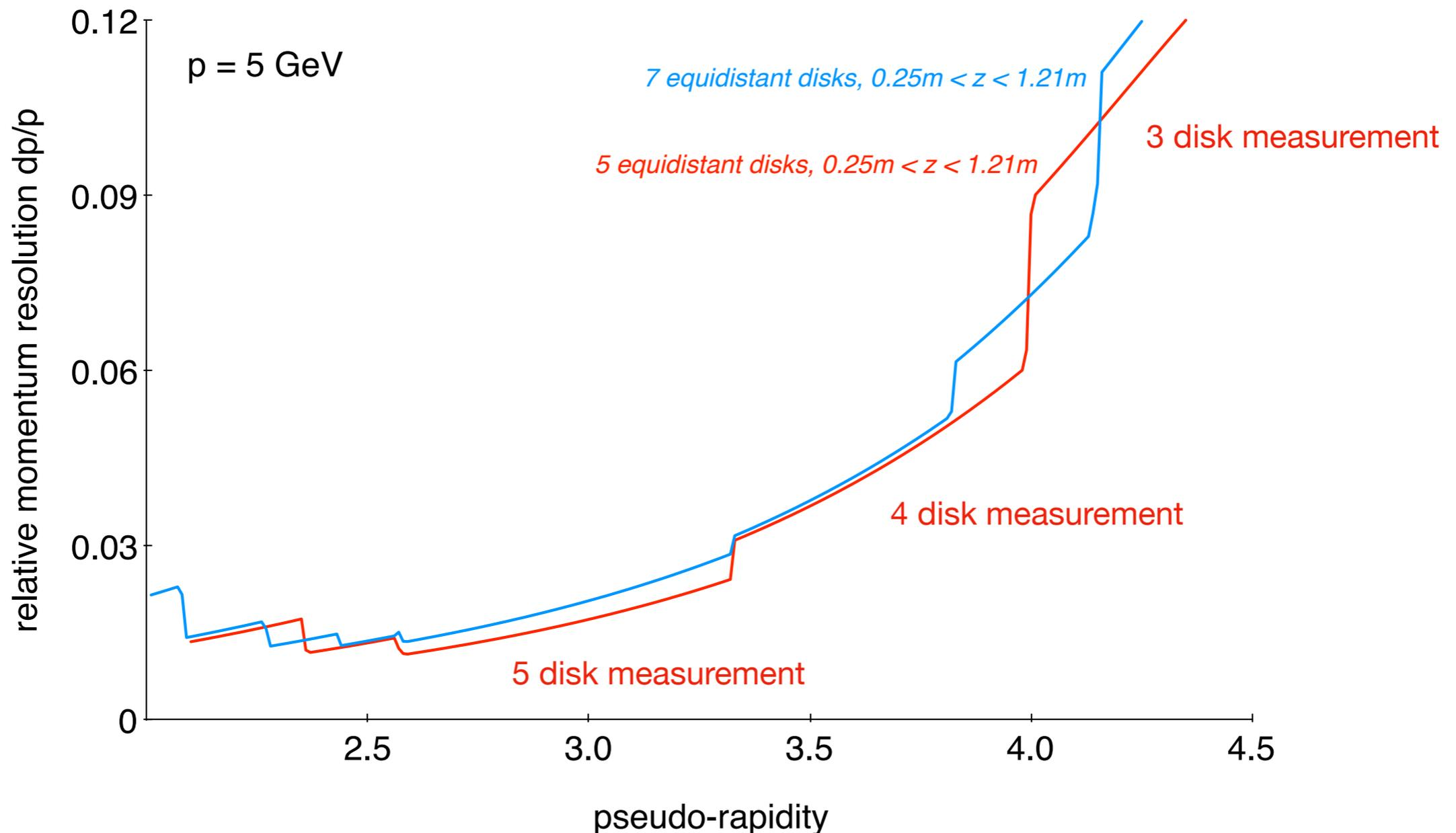
The positions of the steps depend on inner and outer radius; the increased beampipe diameter again enters and impairs large  $|\eta|$ .
