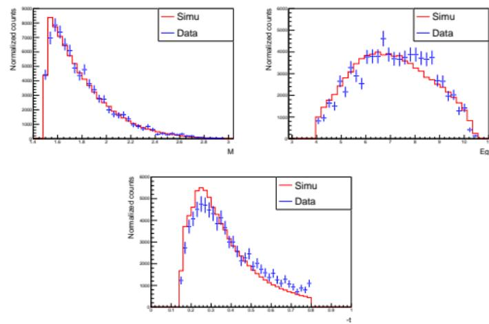
Data/BH simulation comparison in the high mass region  $4 \text{ GeV} < E_\gamma < 10 \text{ GeV}$
