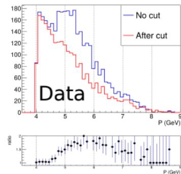
When applied to data and simulation, the pion contamination is removed. The ratio  $B/S$  is reduced from 50% to 5% using the neural network approach (see Back-Up slides for details).
