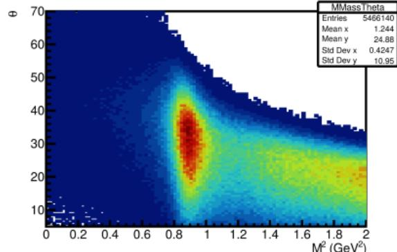
Missing proton mass spectrum; as a function of the missing particle  $\theta$  angle.
