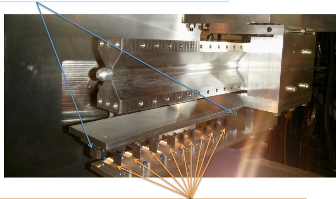
Optical target: a series of foils of carbon (9) to check the alignment of target and spectrometers (optics)
