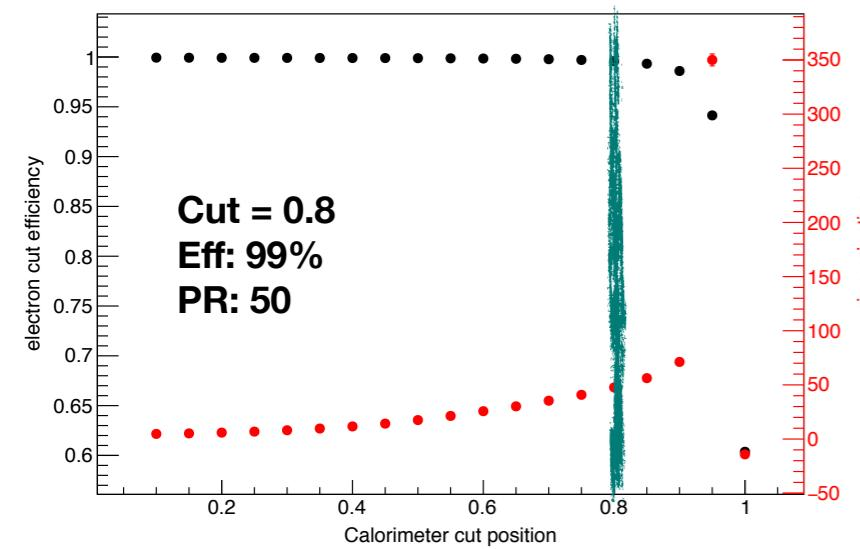
SHMS Calorimeter cut efficiency and pion rejection factor
