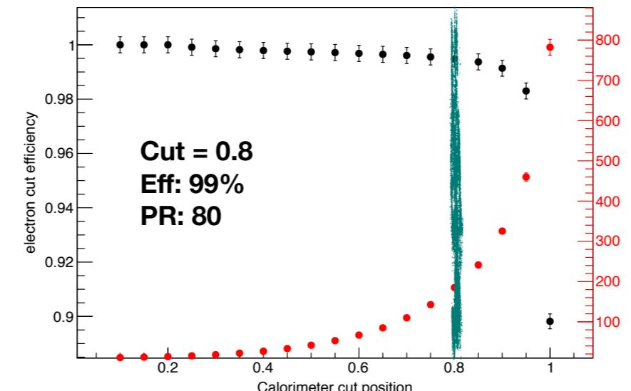
HMS Cherenkov cut efficiency and pion rejection factor
