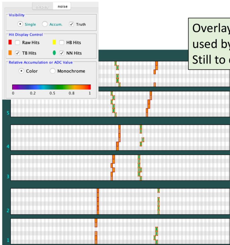
Overlays hits (in greenish color) used by the neural net trackfinder. Still to do: draw the nn tracks.
